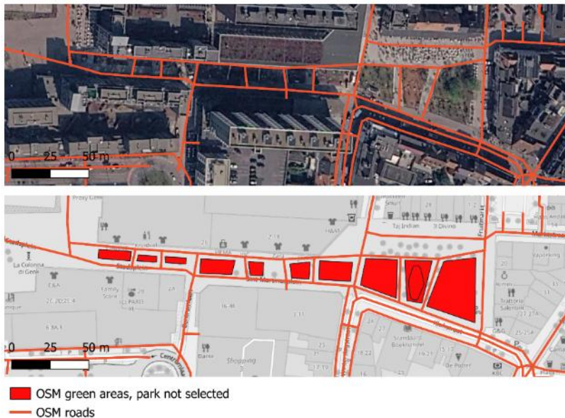
Figure 14. Accessible park in the city centre of Genk, Belgium. Although both the road network and the park are included in the OSM dataset, the roads do not actually intersect the green space polygons. As a result, the green space polygons are, therefore, not considered in the proximity analysis of accessible green spaces.
