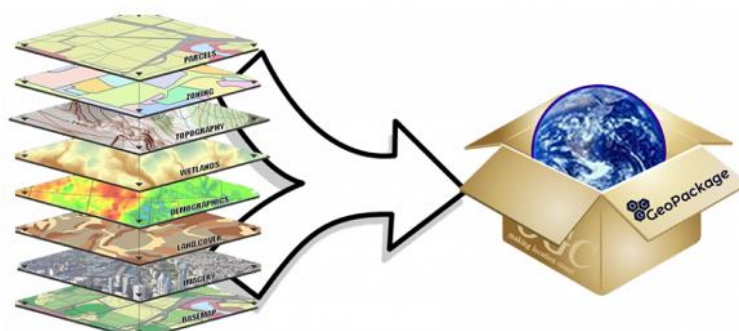
Figure 4.9: Illustration of the GeoPackage file format and one of its key features, i.e., the possibility to store many spatial layers within a single GeoPackage file. 3
